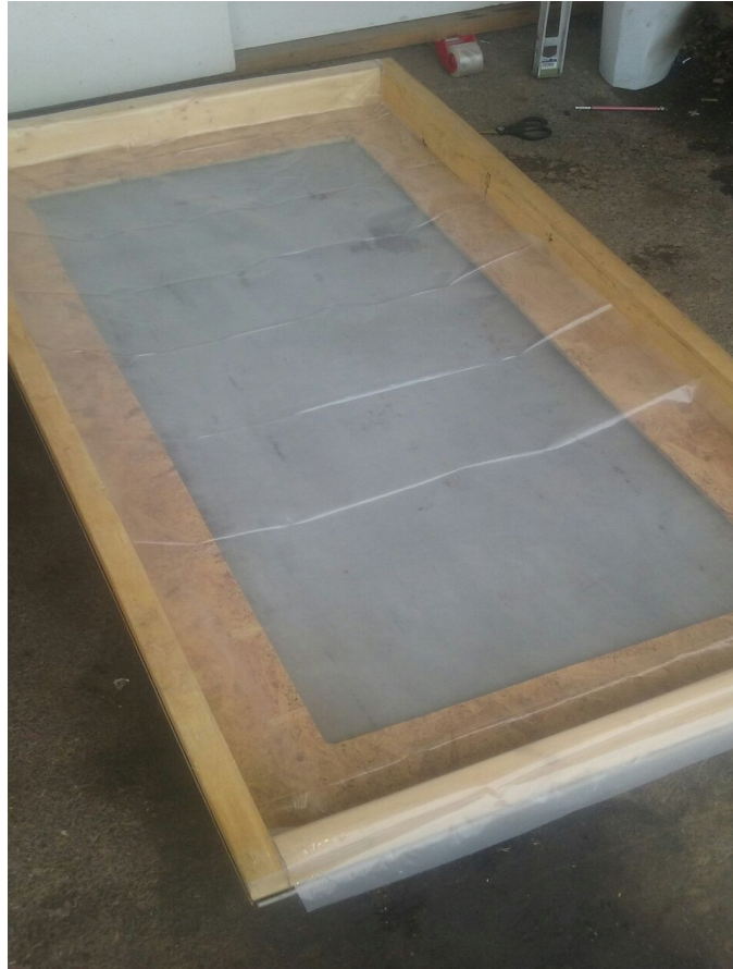
Figure 1: This is a top view of the plug which has a hole cut out so the child torso, head, and arms will be outside of the cart.
