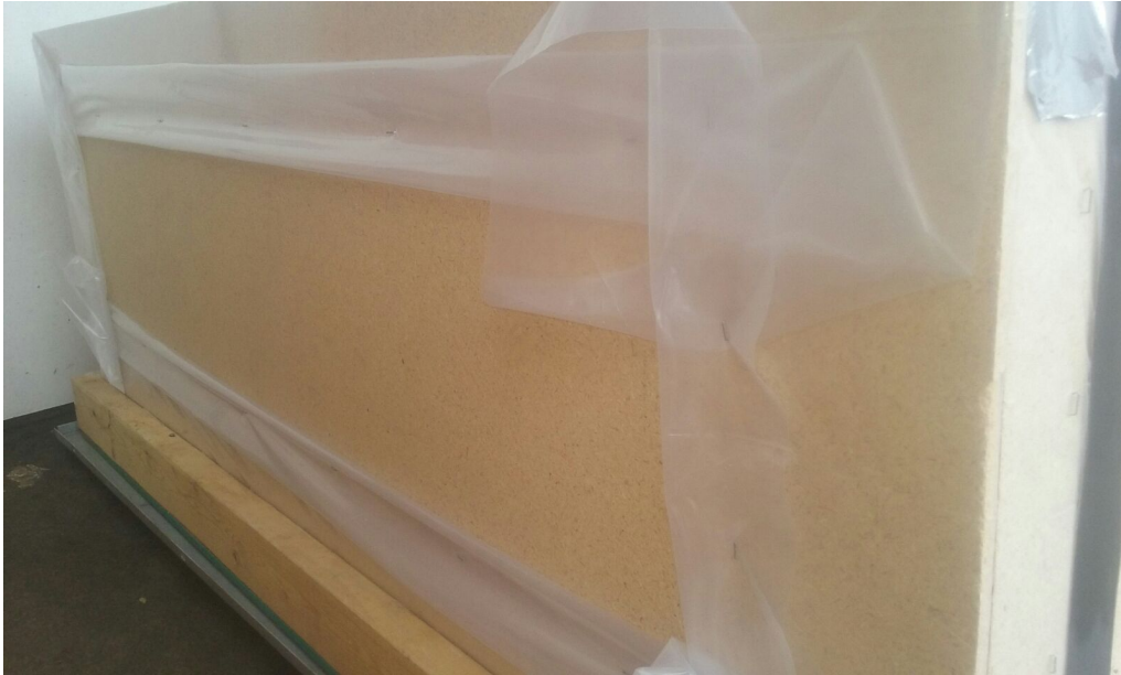
Figure 3: that's an outside look of how the plastic sheets works on one side, and then secured on the other side. Noting that will prevent it from getting contacted with the fiberglass resin.
