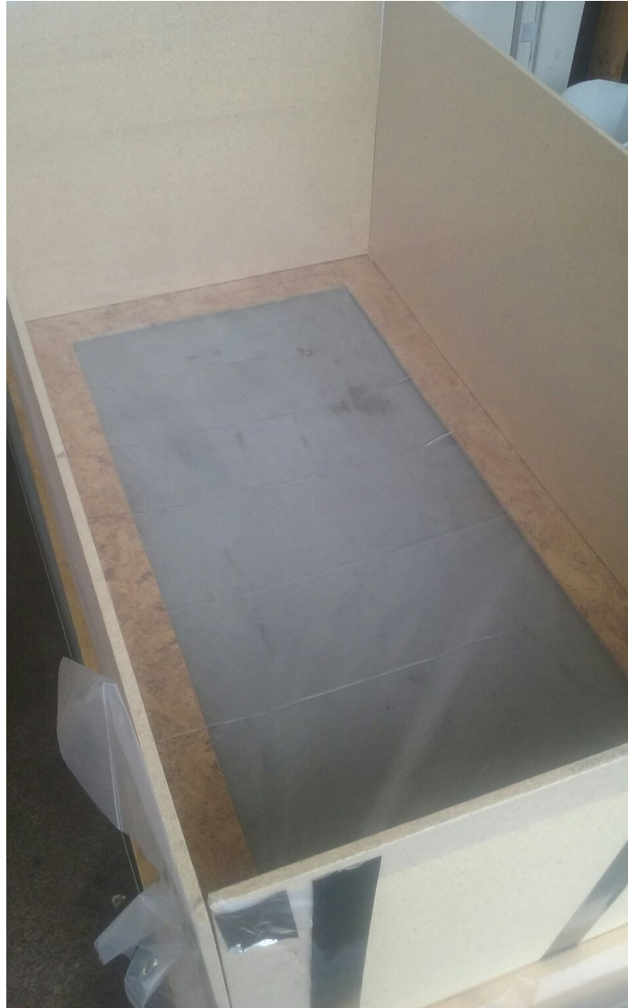
Figure 2: those would be the side walls from wood to get the part ready for molding. Everything is lined with plastic, but it's hard to see. Basically, a plastic sheet is wrapped around every piece of wood.
